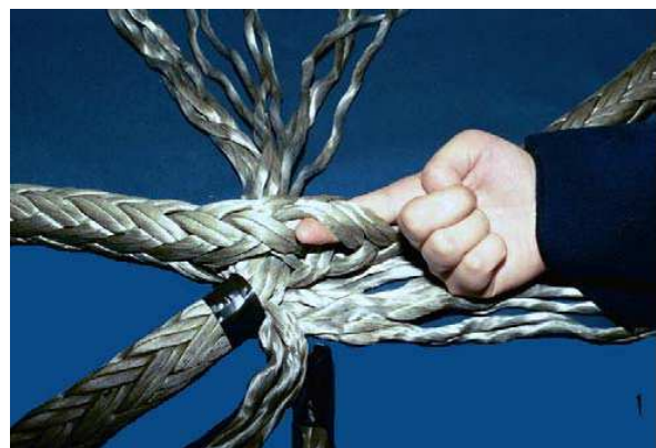
6. Make a hole under two strands in the rope. Choose convenient taped strands to work with and.....
