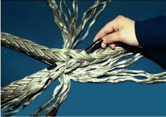
7. ...pull it under the two strands in the rope.
