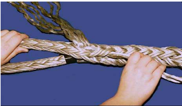
15. The rope is turned over to the other side and the strands spliced into the rope as before.
