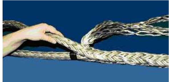
14. Same is repeated for the other strands on same side.
