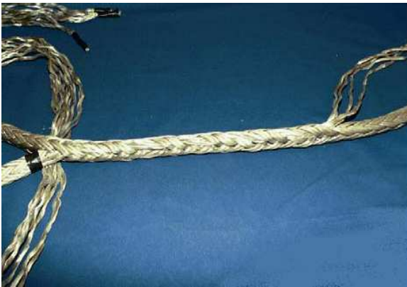
9. Continue this five times so the total times under will be six times.
