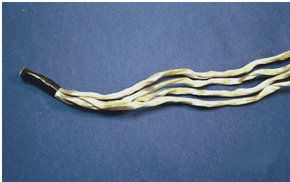
3. The strands taped together should have same twist direction.
