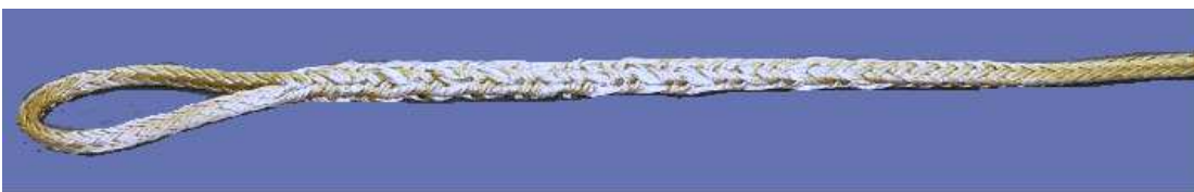
19. The splice is now finished and it should look like this.
