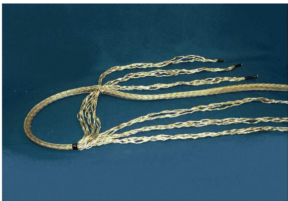
5. Divide the strands in two parts and pull one of them through the opening.
