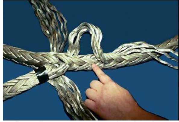
8. Pass then over one strand and again under two.
