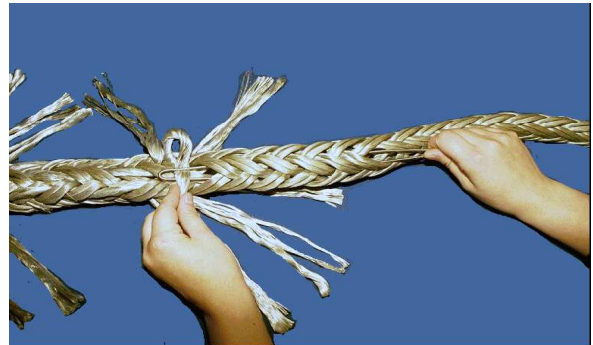
18. The short strand ends are pulled into the centre of the rope.
