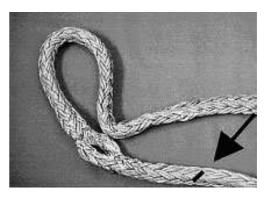
**Step 4**Pull the end all the way through until the rope is through itself.
