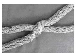
**Step 2**Open the rope where the eye starts to mark the size of the eye.
