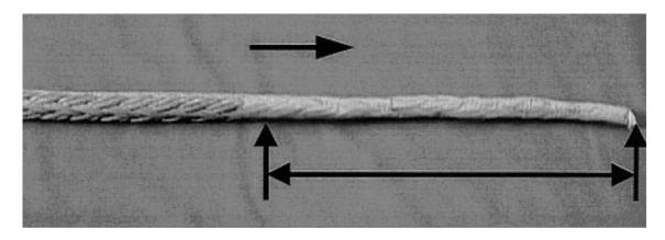
**Step 8**To finish the splice the end is threaded into the centre of the rope. Begin to thread four braidings from the lock.
