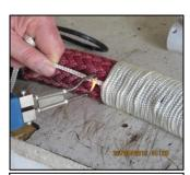
The excess braid can be neatly trimmed.
