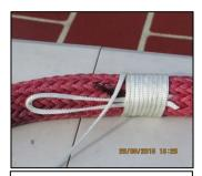
Begin tightly winding nylon braid across the repair section beginning from open loop end.
