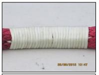
The repaired section is now left to dry. Once dry the braid will be firm on the strop and ready for coating.
