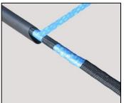
Whilst under tension cover damaged section\* end sections with Masking tape.
