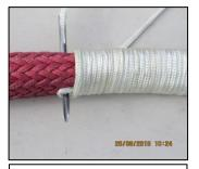
Bring the end of the braid through the Mongoose strop and through the loop.
