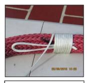
Begin tightly winding nylon braid across the repair section beginning from open loop end.
