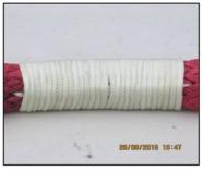
The repaired section is now left to dry. Once dry the braid will be firm on the strop and ready for coating.
