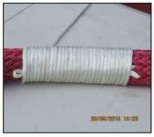
Wrap the braid to the end of the loop fully covering repair section.
