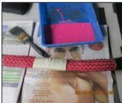
Prepare for coating with Donaghys Urethane Rope Coat with a paint brush to apply.
