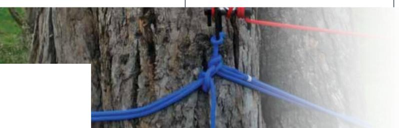
Note: The Australian Fibre Rope Standard AS4142:1-1993 recommends a minimum safety factor for rope sling use of 6:1. (i.e. Ropes subject to occasional flexing or twisting e.g. ropes in made up articles such as slings, tow ropes).
